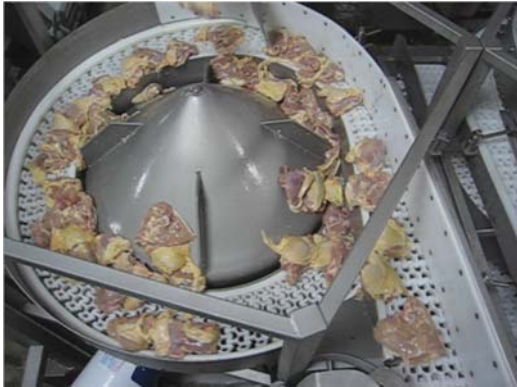
Thighs Metered into the Patented Rotary Singlefiler.
