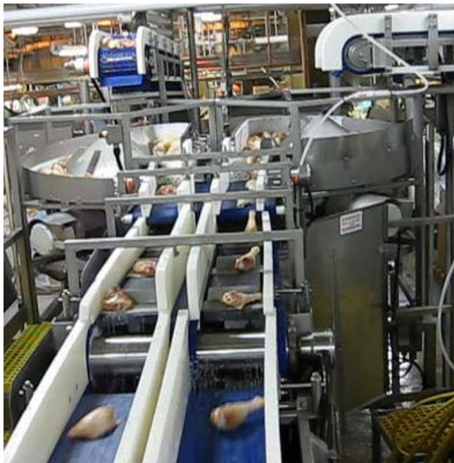
Drums & Thighs automatically singlefiled out of the Rotary Singlefiler. Spacing is attained in the Patented Product Spacing Machine. Side pictures show spacing attained across an in-motion scale and control panel indicating correlating data.
