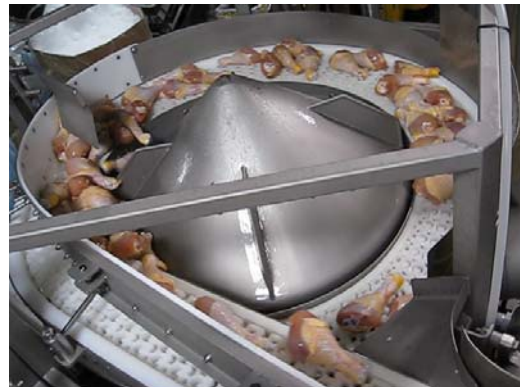
Drums Metered into the Patented Rotary Singlefiler.
